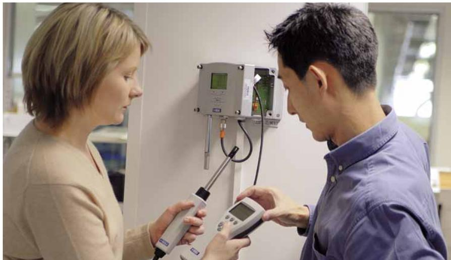
Users often ask manufacturers for a recommended calibration interval. This is a reasonable starting point, but in practice, instrument performance may degrade at different rates depending on the use of the instrument, so the user must establish an appropriate calibration interval.
